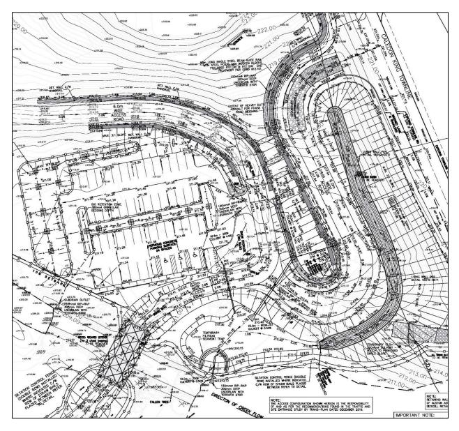
Of note the entrance road required significant design finesse in order to achieve safe traffic movement in accordance with O.B.C and local grading codes while overcoming a 10 metre vertical grade difference between the municipal road and the internal parking areas for the site. The treatment of swales and ditches also required careful attention to ensure no risk of erosion due to the steep grades.
